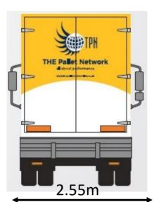
Payload is 9 tonnes. Tail-lift weight max. 1000kg
